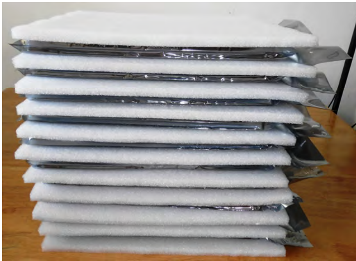
Place Foam Sheets Between Trays
